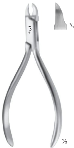
ANGLE EL-D-1513 Wire cutter for soft wire up to 0.5 mm, for hard wire up to 0.3 mm 130 mm, 5 1/8"
