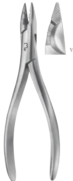
EL-D-1508 Pin- and wire cutters for soft wire up to diam 1.5 mm, for hard wire up to diam 1.2 mm 160 mm, 6 1/4"
